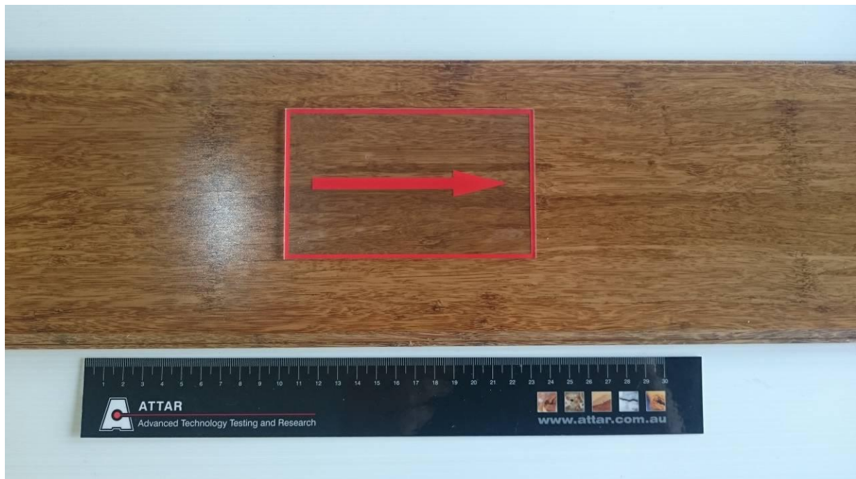
Figure 1: Arc Bamboo Flooring. Highlighted area indicates direction of test.
