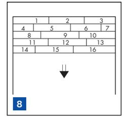
**6** Depending on the width of the room, you may choose to 'rip down' the starting planks, so you are not finishing on the opposing wall with thin pieces. If the starting wall is curved, the first row may need to be scribed to accommodate this. Use spacers! Always cut off the tongue on the first plank also on the short side.
