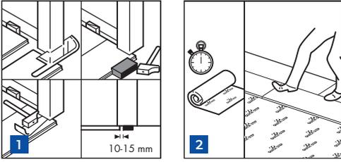
**1** For a nice finish where the next flooring meets a threshold, we recommend undercutting the architrave and door jams. This is best done prior to commencement of the installation. Use a piece of flooring and underlay as a guide, and with a flexible hand saw undercut wherever possible. Then the cut end of the flooring can slide in under the jam and out of sight. The final planks will need to be ripped down the length and brought into position using the pulling bar if necessary.
