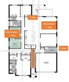
Trowel out enough adhesive to lay out and align the first 2 rows at a time. Ensure that as you layout the flooring along the Y axis that flooring remains aligned as you go. Slight adjustments will need to be made as you go along. Only trowel out small sections of adhesive to avoid adhesive drying out and forming a skin which could reduce adhesion strength. Use the X axis in the same way as to keep alignment of the herringbone pattern.
