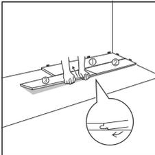
Now place your BOTH hands close to the joint as shown in the figure and pull the long side of the plank towards you.
