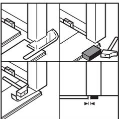
Before you start, it is easier to undercut any door frames using an undercut saw or a flexible blade hand saw and an offset of flooring. Removing the bottom of the door frame and approximately 40mm of adjoining skirting boards allows the floor to expand freely under the door frame and finish neatly at the floor junction. In many instances, the base of trims or profiles to be installed are best installed prior to installing the flooring itself.
