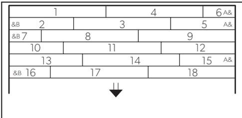
Once enough rows are installed, it is easy to continue the installation as follows: Put an unopened pack of panels on the already installed rows. Switch your position and click the short side of the panel in the previous panel. Now place your BOTH hands close to the joint as shown in the figure and pull the long side of the plank towards you. The panels will now click together. Continue like this to the end of the room.
