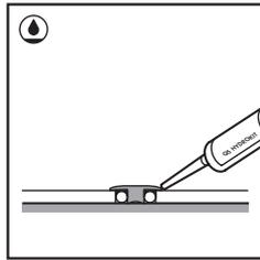
In addition to the floor perimeter, we recommend that the underside of the trim/profile and door jambs or other floor penetrations be sealed using the hydrokit in these wet areas. It is also recommended to separate wet areas where possible using an Incizo trim (i.e. at bathroom or laundry door junctions).
