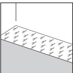
Underlay is essential for all laminate installations. The specially designed Quick-Step underlays have a damp-proof, insulating, noise-reducing and slight leveling function. The smooth top surface makes installing the laminate panels easier and allows the floors' expansion afterwards.
