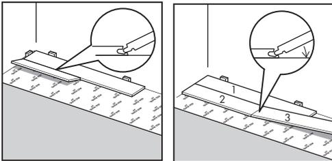
Continue now install the first board in the second row, ensuring that the end (or short) joints of any consecutive rows are at least 300mm apart to create a random staggered appearance and reduce wastage. Continue to install the boards as shown in the pictograms below and remembering to maintain the expansion gap using the spacers. After the first few rows are installed, use the offcut from the last row installed to start the next row.
