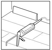
Fix skirting boards or scotia using quality construction adhesive and/or brads or small diameter nails. It is important to never attach or glue the skirting board or scotia trims to the floor. This method allows the floor to expand and contract under the profile.
