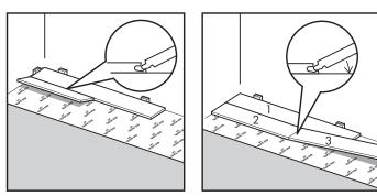
Continue now installing the first board in the second row, ensuring that the end (or short) joins of any consecutive rows are at least 300mm apart to create a random staggered appearance and reduce wastage. Continue to install the boards as shown in the pictograms below and remembering to maintain the expansion gap using the spacers. After the first few rows are installed, use the offcut from the last row installed to start the next row.
