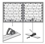
There must also be at least a 10 mm expansion joint between the last row and the wall. Keep this in mind when sawing the last row of panels.
