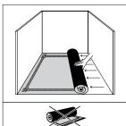
Remove any damp-open floor covering (carpet, needle felt, etc.) first. Damp-proof floor covering (PVC, linoleum, etc.) does not have to be removed. Always use an underlay. We recommend the use of Quick-Step Combi-Lay or Quiet-Step Combi-Lay. These underlays provide a very high damp performance of SD> 75m. If an alternate underlay is to be used, ensure it achieves at least an equal damp performance, otherwise irreparable damage may occur.
