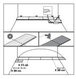
Of course you also need to saw the panels. To obtain a clean cut, a downwards cutting jigsaw blade should be used or the top surface should face down when you use a jigsaw, or circular handsaw and up when you use a handsaw or a crosscut saw. Ensure that the end joints of the panels in two successive rows are never in line. Always ensure that the joints are staggered by at least 15 cm.
