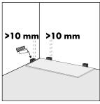
Put the plank with sawn off sides against the walls. Put spacers from the installation kit between the planks and the wall. This will ensure that your expansion joint is wide enough. Remember, depending on the relative humidty the floor may require more room to expand or contract than the standard 10mm. In areas of high humidty like northern coastal Queensland, Australia, up tp 14mm perimetre expasion gaps may be required.
