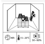
Packaging should be opened and planks allowed to acclimatize for 48 hours prior to installation at the normal room temperature, in the middle of the room where the floor is to be installed. The ideal conditions are 15-20°C (59-68°F) at a relative humidity of 50-60%.
