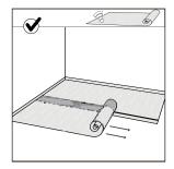
First lay the underlay across the breadth of the room and then gradually as you lay the planks.
