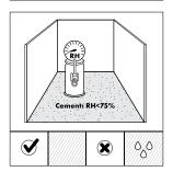
Fresh screed must dry for at least 1 week per cm thickness up to 4 cm and 2 weeks per cm thickness over 4 cm, with sufficient ventilation. For example, a 6 cm screed must dry for at least 8 weeks. For the thickness over 6 cm you must add 3 to 4 weeks. The relative humidity of the concrete should not exceed 75% RH when tested in accordance with AS1884-2012.
