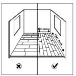
Always lay the product down the length of the room to minimise the running LM in the width.
