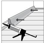
Install the skirting-board. Never attach the skirting-board to the floor. This method allows the floor to expand and contract under the skirting-board.
