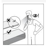
Inspect all planks in sufficient light before and during installation. Planks with visible defects must never be used. Proceed with a visual inspection of the planks before installation. Once installed, the planks are considered accepted by the installer and owner.
