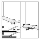
Position the panel to be installed at an angle of 20 to 30° to the panel already laid. Move the panel gently up and down and at the same time exert forward pressure. The panels will automatically click into place. Position the Uniclic tapping block over the short joint between the panels and tap carefully until the panels fully align.
