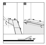
Click the first panel of the second row in the previous row. Click the short side of the panel in the previous panel. Then lifting the panel 20-30 degrees up along the length of the panel, gently tap the panel together with the previous row using a Uniclic tapping block and hammer.
