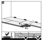
Tap the cross joint between these panels snugly together using the Uniclic tapping block. Make sure both panels are level on the subfloor and that you position the tapping block as indicated in the diagram to avoid damage.
