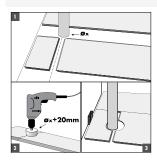
In rows where there is a pipe, make sure the pipe falls exactly in line with the joint between two panels. Take a drill bit with the same diameter as the pipe plus 20 mm. Click the panels together on the short side and drill a hole centred on the joint between the two panels. Now you can install the panels on the floor.
