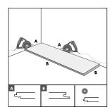
Begin the first row with a whole plank. Saw off both the long and the short tongue from the first panel.
