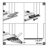
When sawing the panels ensure that the expansion joint under the door is at least 10 mm. If you cannot lift the panel, use an adapted tapping block or crowbar and hammer to tap the panels together.
